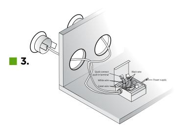
Connect the wires of step lights to the wire of the driver in the junction box. The max quantity of the step lights depends on the wattage of the driver.
