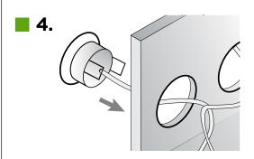
Push spring-loaded clips on the step light upwards and insert the fixture base into the mounting hole. Release the clips and the fixture will be pulled flush to the wall.
