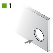
Determine the location for installation and cut a hole on the wall with dimension  $\emptyset$  1-3/4".
