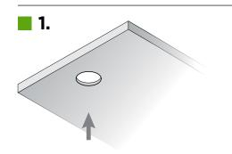
Determine the location for installation and cut a hole on the bottom of cabinet with dimension Ø 1".
