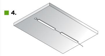
Connect the first light bar to the connector from the junction box. Then connect the other light bars to the previous light bar one by one. The max wattage showed as below.
