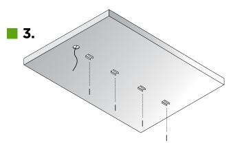
Install the stain steel clips with the little screws to the bottom of the cabinet. It needs 2 clips to hold each light bar and make sure they are on the straight line.
