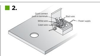
Put the junction box in the cabinet. The most important thing is to make sure it is CLASS II power and the output voltage is DC12V. Open the junction box cover and remove the appropriate knockout(s) on the side panel. Insert the electrical supply cable through the knockout and secure with a cable connector (sold separately).
